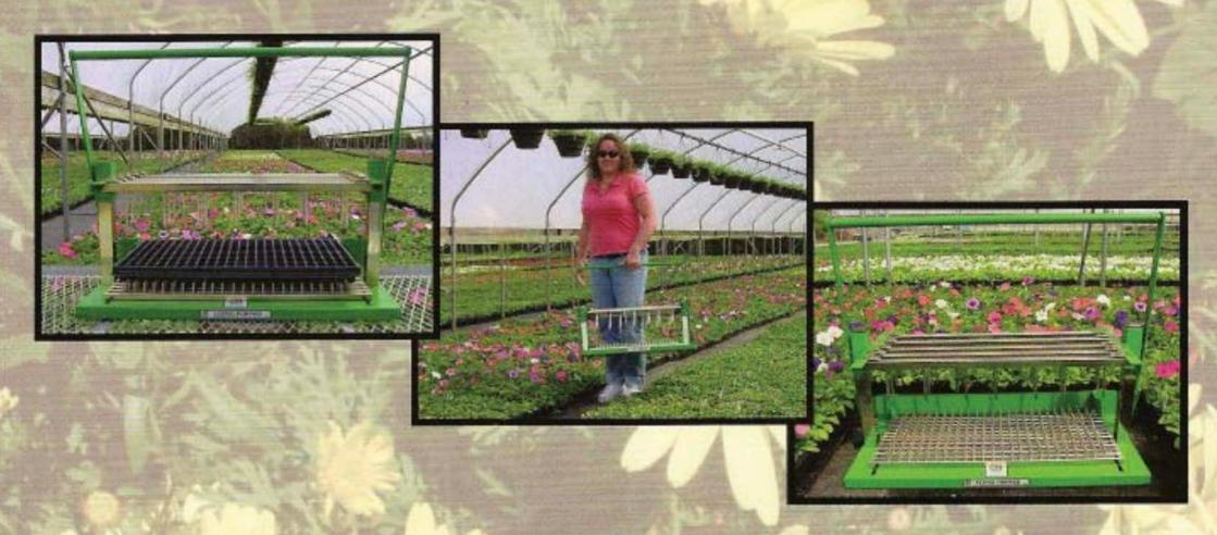
The "Econo Popper" is the first universal, hand-operated, portable dislodger. At only 40lbs, it's easy to transport between workstations. The unique pin lock system allows the extraction and hold down pins to be adjusted to fit virtually any standard 10" x 20" tray.
