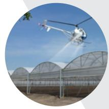
For the best crop result, a coating must be applied to the greenhouse cover as evenly as possible. An uneven layer may cause growth differences in the crop. The weather during application also has an impact on the result. The coating must have enough time to dry but drying too fast produces a suboptimal result.
